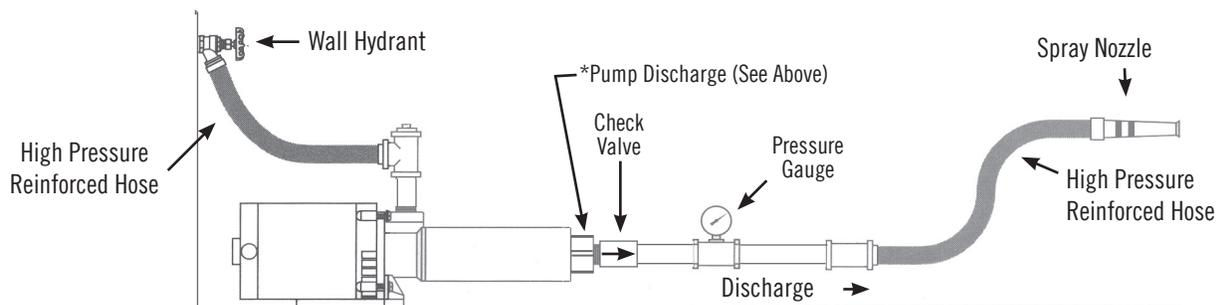
Whenever a spray nozzle is used, a pressure switch should be installed to automatically turn the pump on and off. This eliminates the possibilities of operating the booster pump at shutoff pressure, which could damage the pump due to high temperatures.
