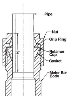
6. The maximum sealing pressure for these fittings is 150 PSI.
